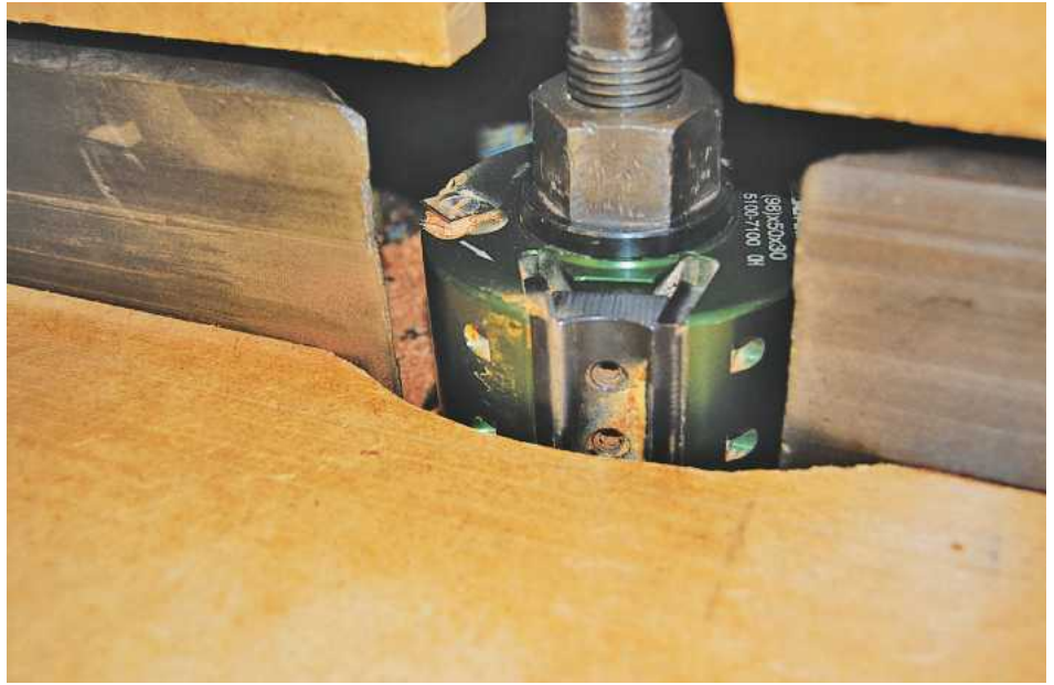
▲ Pic 3 Here you can see the rebate block in the spindle moulder. This was used for the final job, to cut the glazing beads that would hold to glazing units in place...
